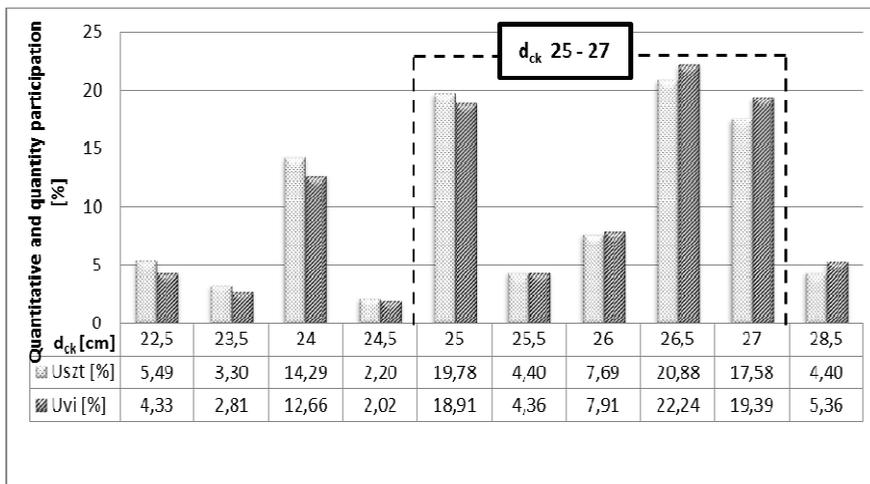
Figure 4. Results of logs sorting acuteness with  $d_{ck}$  25-27 cm (quarter 17) at automatic manipulation line for un-worked logs.
