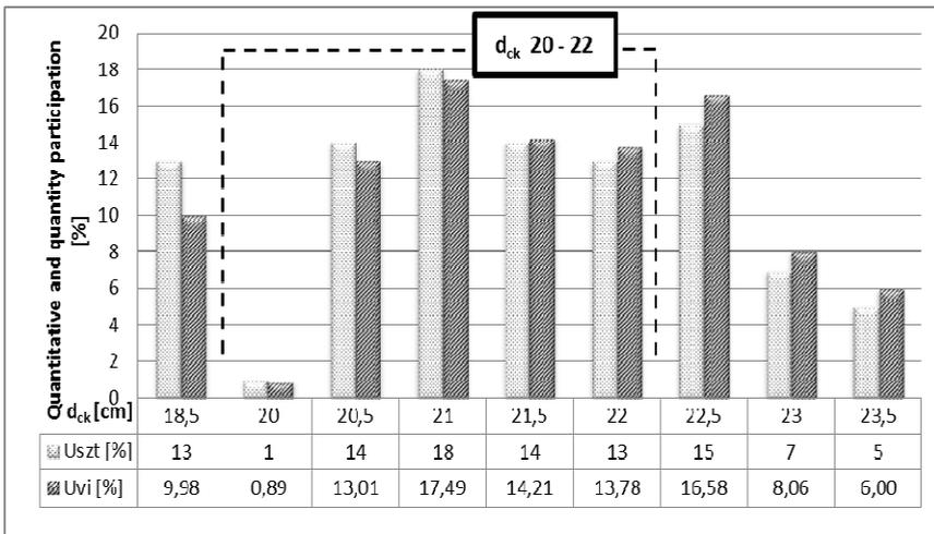
Figure 2. Results of logs sorting acuteness with d<sub>ck</sub> 20-22 cm (quarter 16) at automatic manipulation line for un-worked logs
