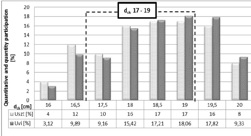
Figure 1. Results of logs sorting acuteness with d<sub>ck</sub> 17-19 cm (quarter 39) at automatic manipulation line for un-worked logs
